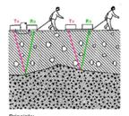
Emitting electromagnetic pulses and receiving reflected signal response. Transmitter (Tx) and receiver antenna (Rx) are pulled as a unit over the survey area.
