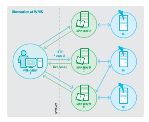
An optional third operation (GetFeatureInfo) provides access to information about displayed map features. With this option the features 'behind' the map can be queried, and their properties can be returned to a requesting client i.e. the user selects a point, line or polygon feature on the map to display further information about that feature.
